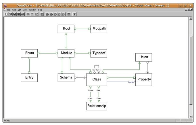
The boxes represent classes, and the arrows are relationships. The ends contain both the relationship labels and shapes that indicate the type of relationship. The bubbles are parent pointers, the light arrows are simple pointers, the full arrows are linked lists of some sort, and the empty boxes are hashed relationships. Arrays would be draw as boxes with an 'X' in them. Light green relationships are cascade delete, and dark green ones are mandatory.
